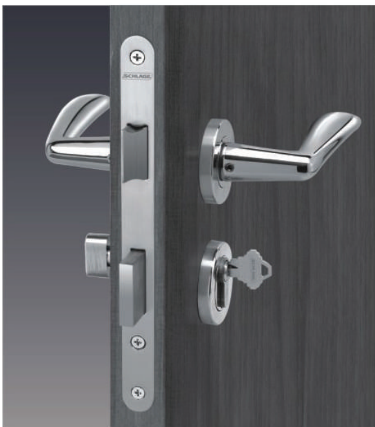
EL2020 Sash Lock Latch bolt retracted from both side by lever handles. Deadbolt is operation by key outside, and by key or thumb turn inside depending on the cylinder selected. The cylinder to latch function enables the cylinder to withdraw the deadbolt on the first turn and the latchbolt on the second turn
