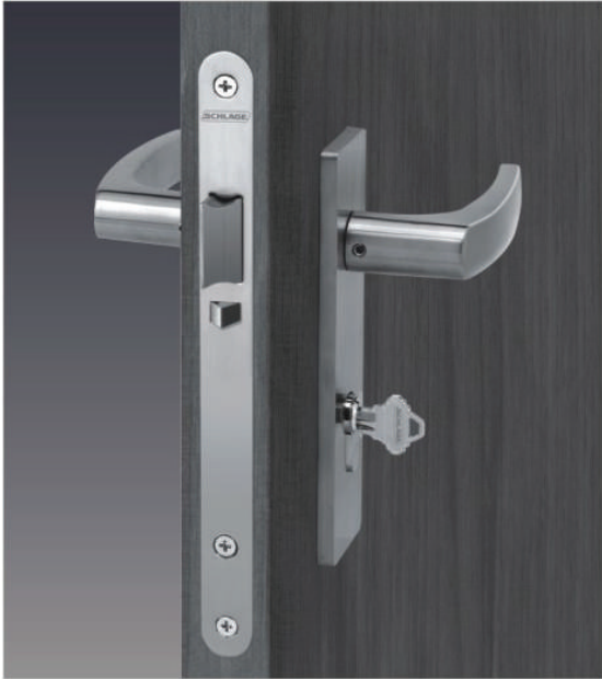
EL2050 Night Latch Latch bolt retracted by key outside or by lever inside. Outside lever always in-operative. Guard latch deadlocks latch bolt when door is closed.
