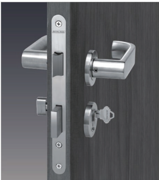
EL2060 Panic Lock Lever handles withdraw the latch bolt from both sides. The deadbolt can be thrown and withdraw from one or both side as required depending on the cylinder selected. From inside, The lever handle will withdraw both the deadbolt and the latch bolt simultaneous.
